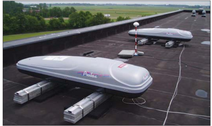
Boxes containing cosmic-ray detectors on a school rooftop as part of the HISPARC project. (Photos courtesy Ilka Tánčzos.)
