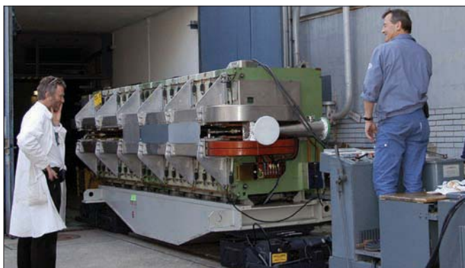
A 35-tonne dipole from the PS is transferred by the 45-year-old locomotive that was brought back into service for the renovations.
