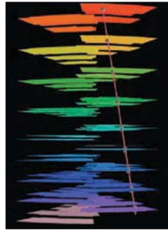
One of the muon events recorded in the first sector of the TEC+, under test in Aachen. The display shows the individual silicon-strip modules in the 18 “petals” that make up the sector.
